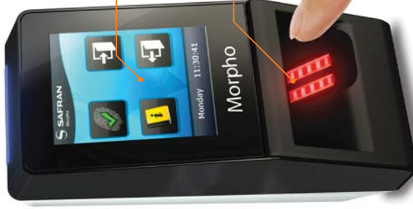
MA SIGMA Lite+ With 2.8" QVGA color touchscreen and buzzer
